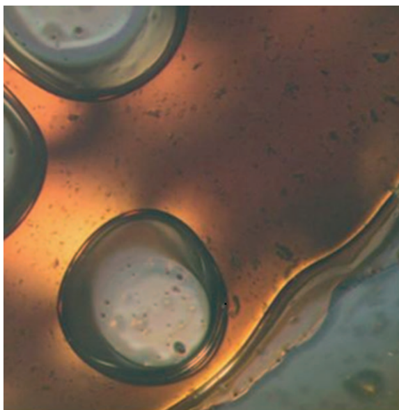
Figure 12. B9-PLM (200 \times ): After 1 h at 250 ^{\circ} C, the compound shows a strong reflection of polarized light. [Color figure can be viewed in the online issue, which is available at wileyonlinelibrary.com .]
